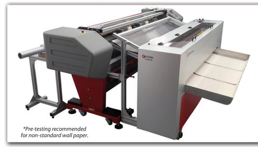
The Fotoba Coreless Rewinder creates a fully automated solution for all wall paper cutting and rewinding applications. It is the perfect solution to cut and rewind media up to 64" wide. This complete finishing package offers quick turnaround times allowing wall paper to be delivered to your customer in a timely manner.
