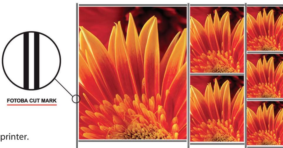
**Regardless of any slight misalignment, when paper is introduced into the Digitrim, the cutter will automatically re-align itself to the image**
